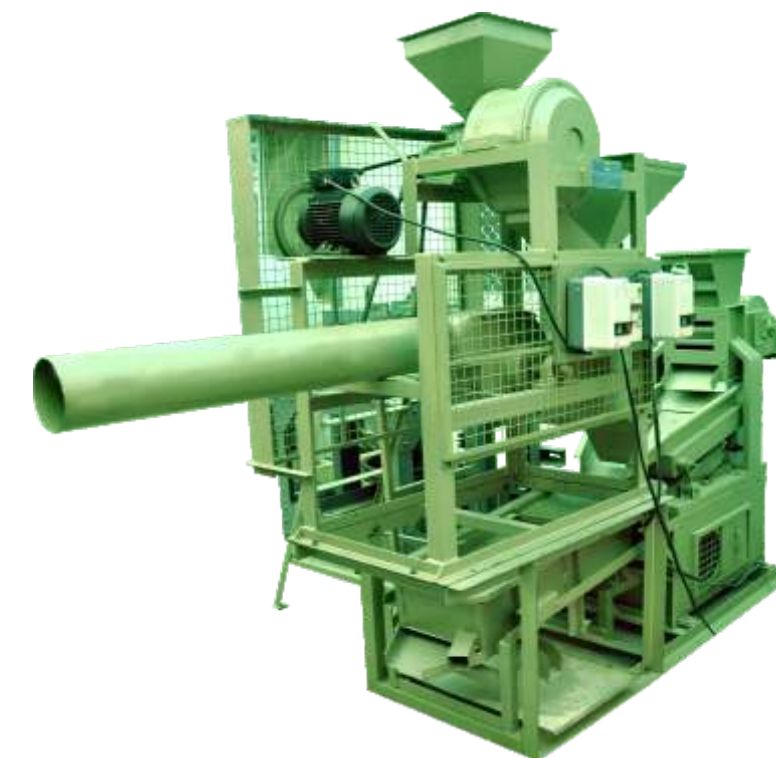
Fig. 5: Small millet destoner, grader cum dehuller
