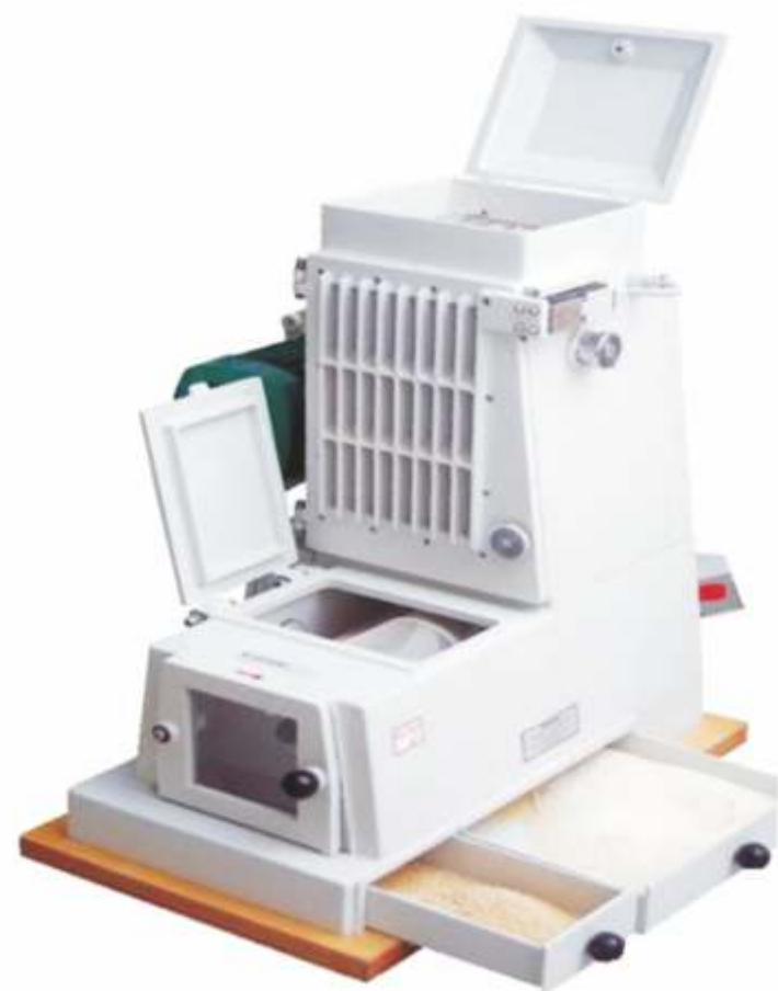
Fig. 7: Fine semolina making machine (Barbender junior)
